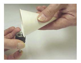
4. Hold the cylinder vertically in one hand with the small end down and resting on a finger tip. Fill the cylinder to the top with clean water.
