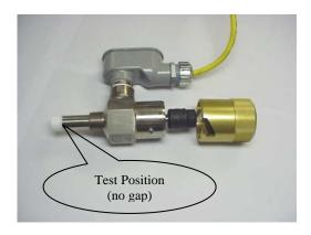
2. The test water injection pump has two sections that are insulated with black plastic shrink wrap. Rotate the larger section (not the one closest to you) ¼ turn counterclockwise and then pull outward to remove the entire pump assembly.
