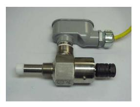
If the signal is not received, the probe has failed the test.
