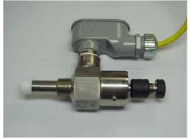
6. Insert the small end of the cylinder to connect it to the probe assembly and rotate the cylinder only (larger section) ½ turn to engage the bayonet pin. Caution: Never attach the water pump if the piston is not installed. Fuel will be released.
