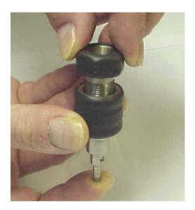
5. Insert the piston and rotate it into the first thread of the cylinder. There will now be 1 cc (l ml) of water in the cylinder for performing the test.
